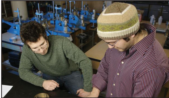
Research assistants Gabriel Iltis (left) and Jesus Higuera Seda (right) working on the preparation of specimens of expansive soil-rubber (ESR) mixtures for swell-consolidation testing.
