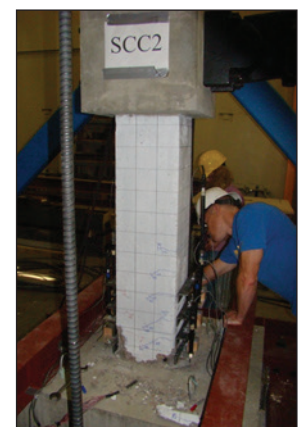
Column specimen during the test
