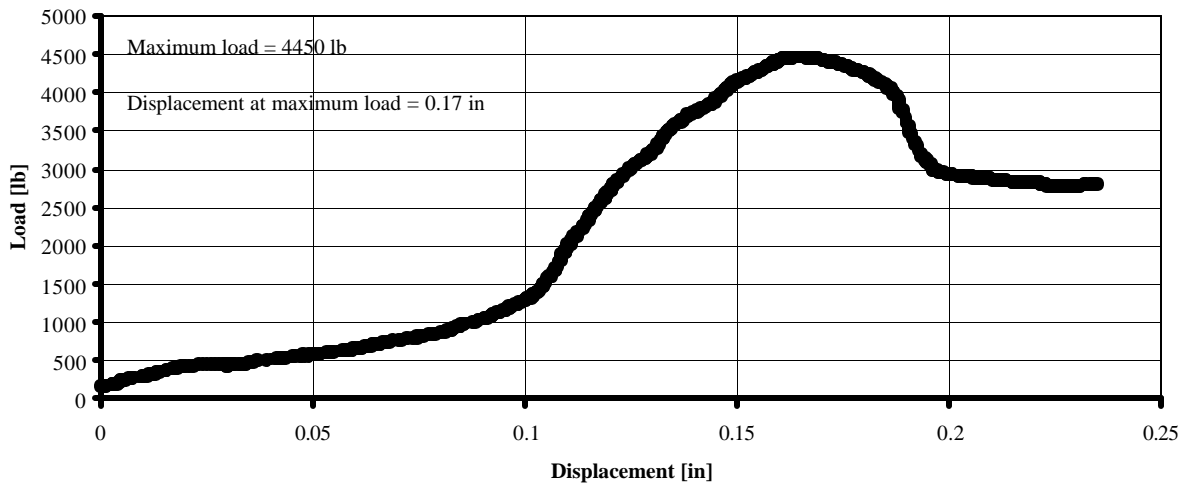
Figure 4.3 – Sample load slip plot for Hilti adhesive with tapping the holes.
