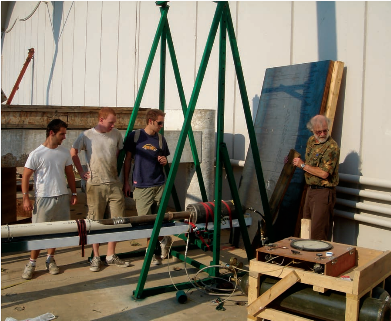
French students look at a cannon for a hurricane impact test.
