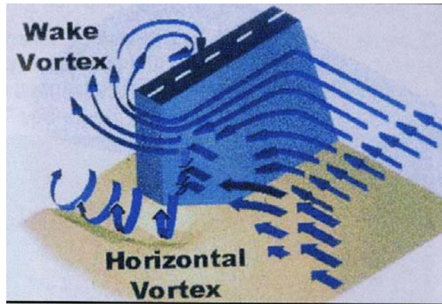
Figure 3. This sketch portrays an unrealistic, or at least very uncommon, view of abutment scour; taken from NHI (2009) "Stream Instability, Bridge Scour and Countermeasures"
