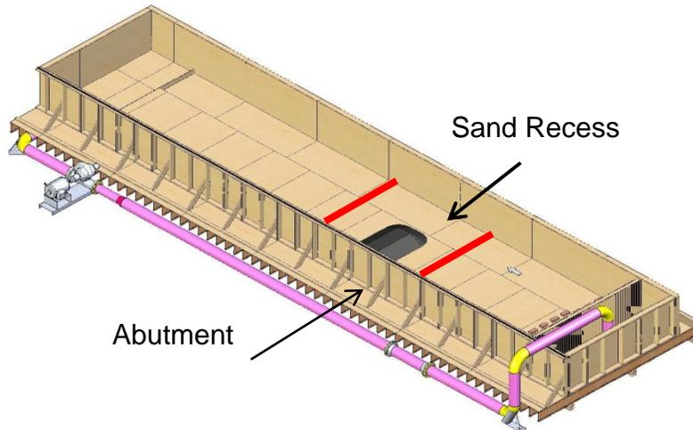
*Figure A-2. The water re-circulating flume at the University of Wyoming, showing the test abutment (black) and the outline of the sand recess that will be subject to clear-water scour (for an abutment sited on a floodplain). Flow is from the reader's right*
