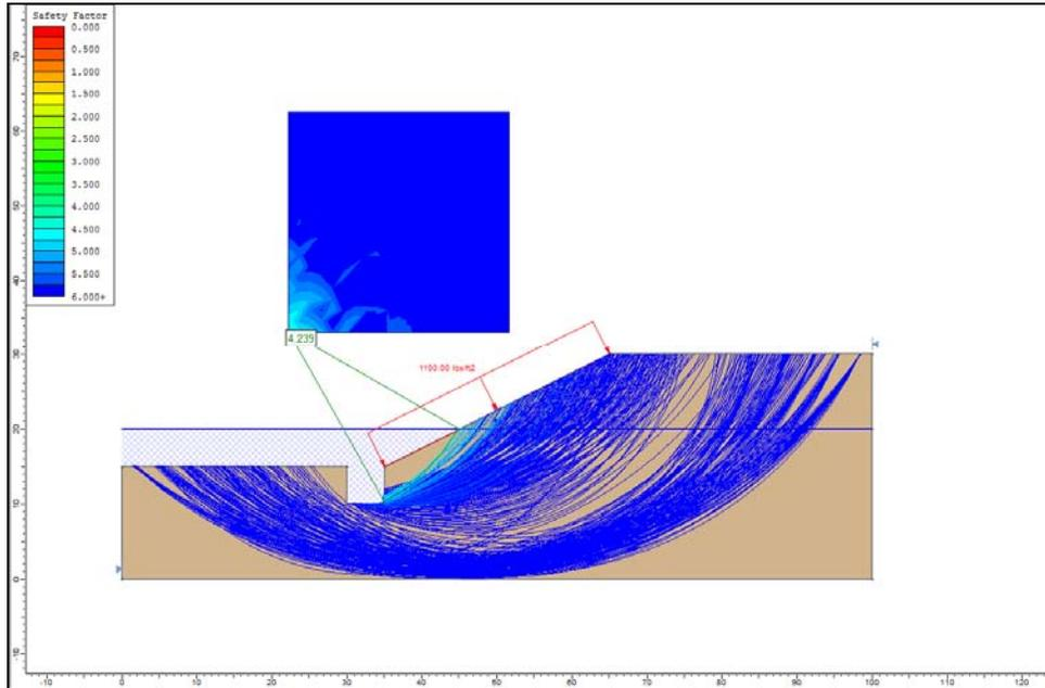
*Figure A-1. Slip failure surfaces calculated using the Rocscience software **Slide (4.0)**. For the spill-slope configuration, riprap layer (represented as a uniform load on the spill-slope), and example scour depth depicted, the spill-slope remains stable at the pre-selected scour depth. However, a deeper pre-selected scour depth may result in spill-slope failure (i.e., a safety factor less than 1)*
