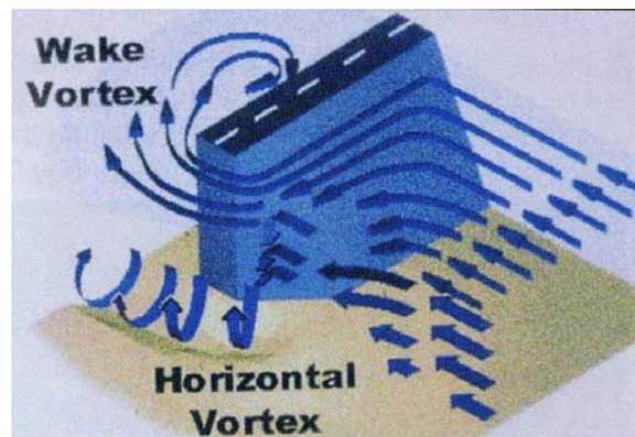
Figure 3. This sketch portrays an unrealistic, or at least very uncommon, view of abutment scour; taken from NHI (2009) “Stream Instability, Bridge Scour and Countermeasures”
