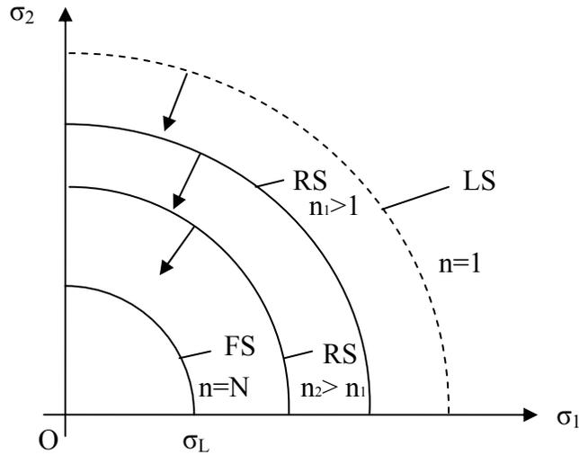
Figure 1. Schematic representation of Strength surfaces in two-dimensions.
