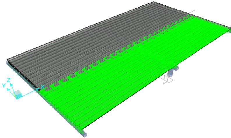
Fig. 1 SAP-based finite element model
