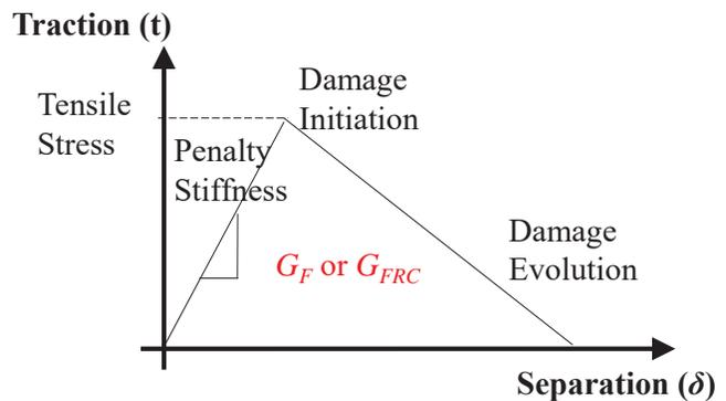
Traction-separation relation for linear softening curve
