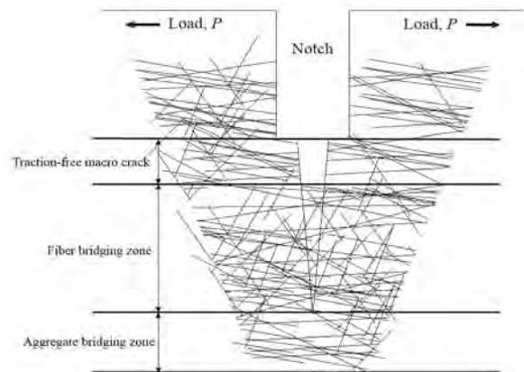
Schematic representation of fibers bridging across a crack
