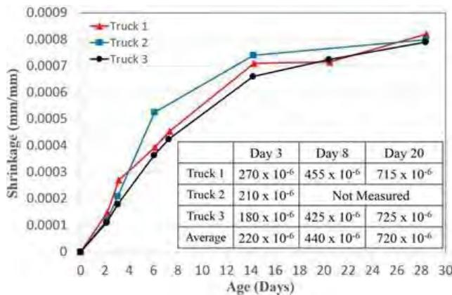
Samples taken during construction to measure the free drying shrinkage
