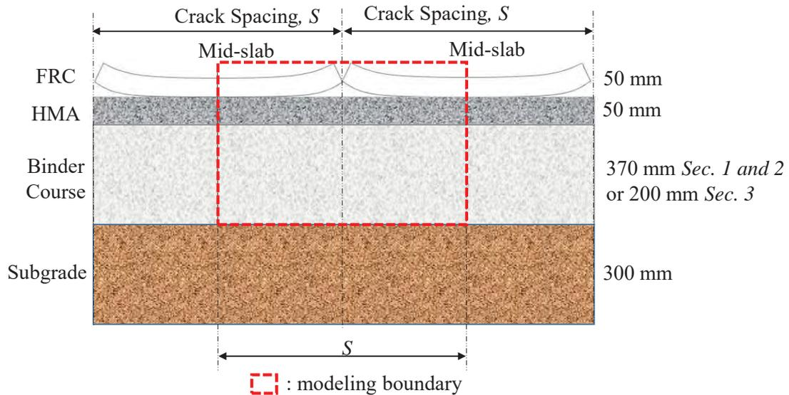
The modeling is simplified because this study focuses on cracking and debonding in FRC layer. The subgrade was idealized using elastic foundation (the stiffness of elastic foundation is 150 kPa/mm).
