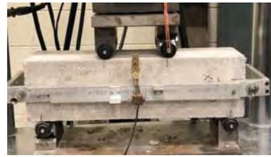
ASTM C1609 test, courtesy of Univ. of Illinois
