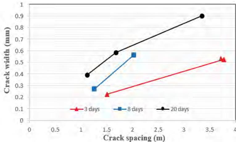
Relation between crack spacing and crack width in FRC overlay
