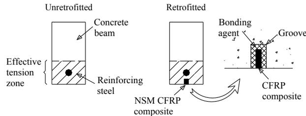
**Fig. 1.** Concept of NSM CFRP-retrofit (Kim and Rahman 2010)
