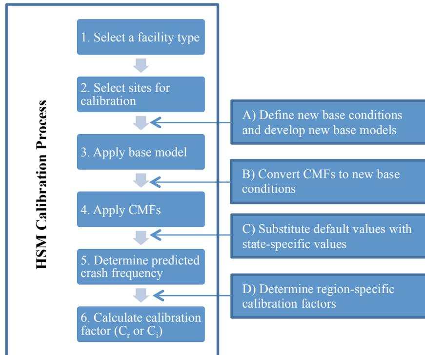
Figure 1. Proposed modifications to calibrate HSM Part C predictive methods.
