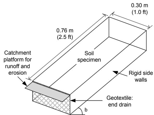
Fig. 2. Schematic of the laboratory-scale slope model to evaluate ground treatments.
