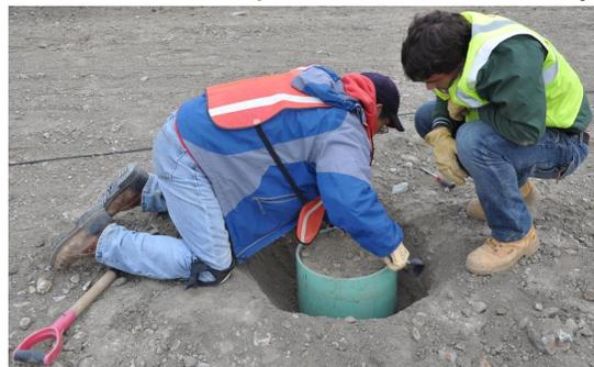
Fig. 1. Photograph of block sampling method; 0.3-m-diameter sample.
