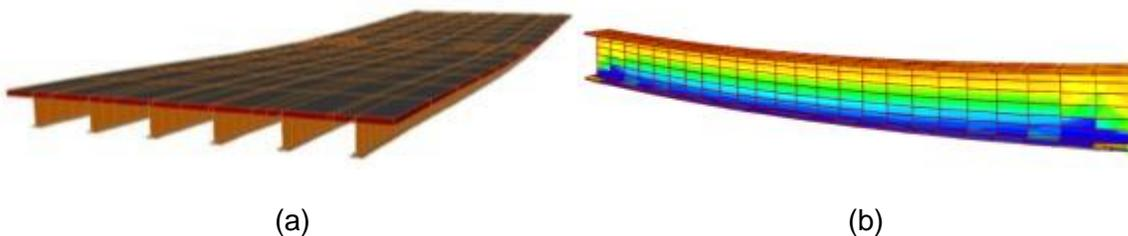
Fig. 2 SAP2000-based finite element models (a) bridge model and (b) thermal analysis on a beam using shell elements.
