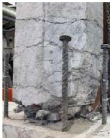
removal of previous CFRP donut (PC1-R2)
