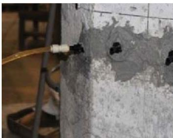
epoxy crack injection (PC1-R2)
