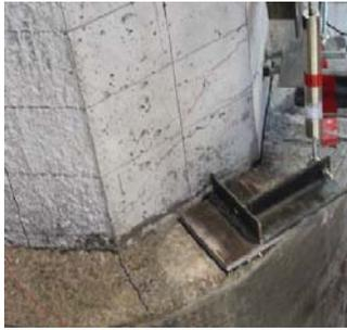
Gap between column and CFRP donut at 2% drift ratio
