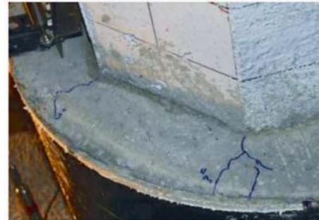
Radial cracks in repair concrete (NM-R1)
