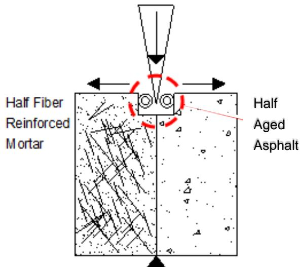
**Figure 2. Interfacial Bond Test using the same wedge-split test apparatus with half FRC and half asphalt.**
