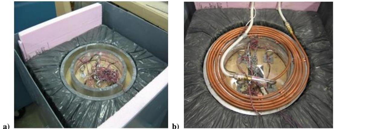
**Figure 1. Dual-Ring Shrinkage a) insulation box with rings ready for mortar to be cast, and b) heating/cooling coil unit on top of cast mortar sample.**
