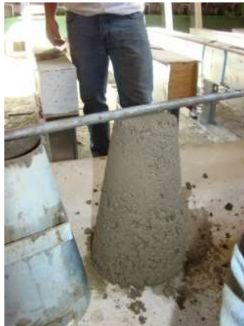
Figure 1 Slump Test: (a) SCC and (b) CC [Error! Reference source not found.].
