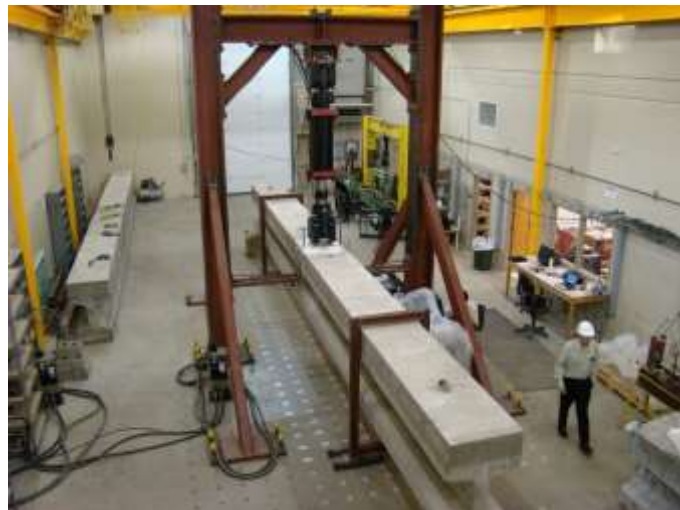
Figure 3 Testing of Representative Prestressed SSC Bridge Girder at SDSU [Error! Reference source not found.].
