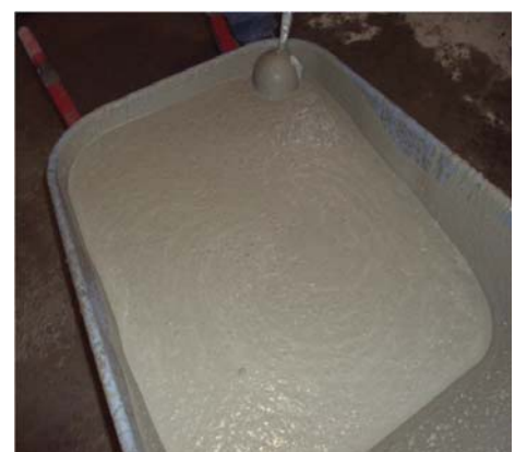
e) SCC showing segregation
