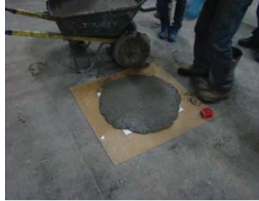
b) Slump Spread
