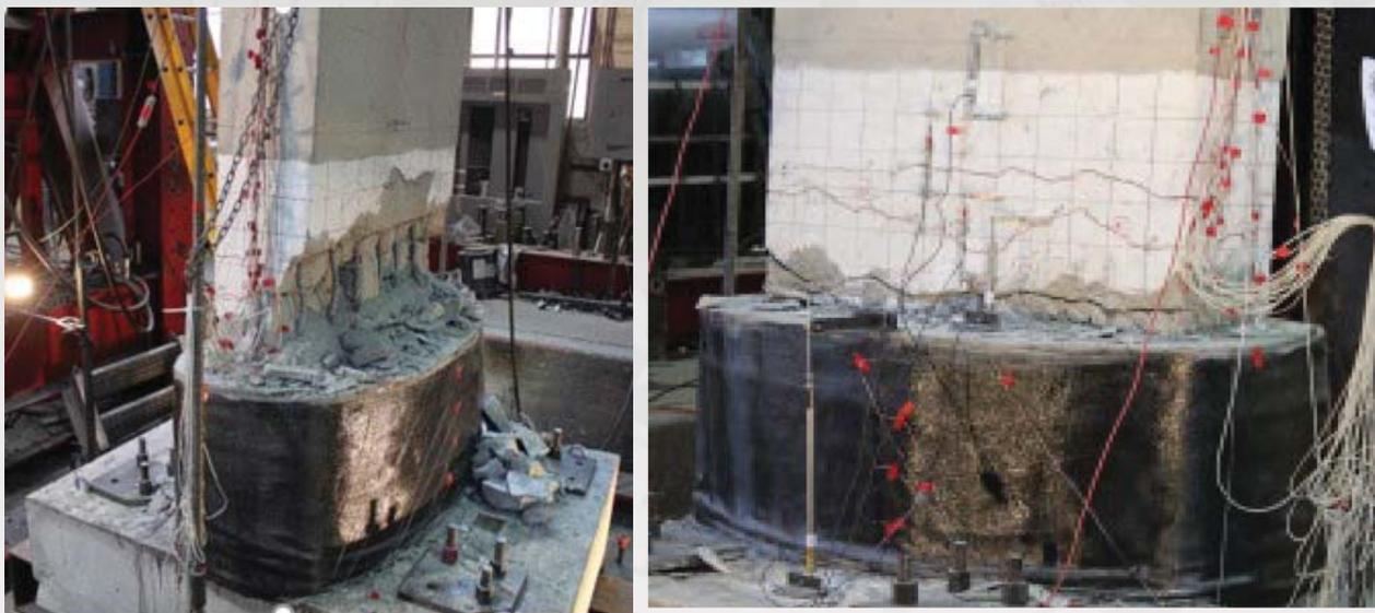
Failure of repaired modern code compliant wall pier: 6% drift ratio
