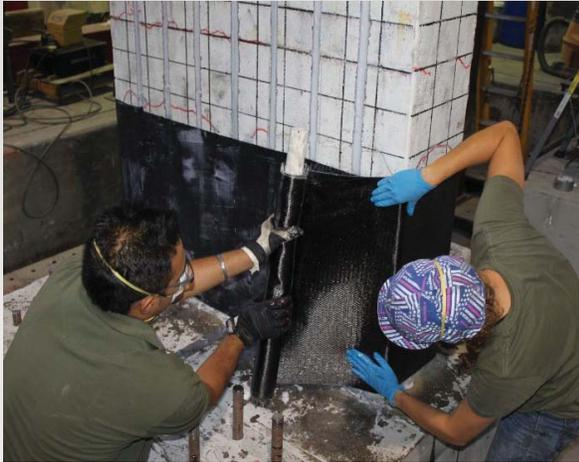
Application of CFRP hoop layers
