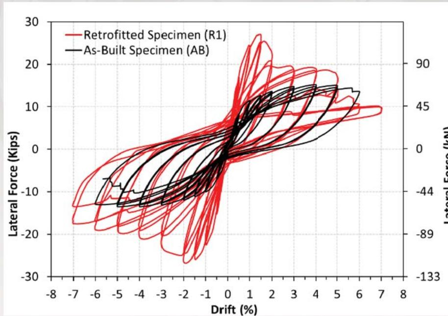
Comparison of hysteresis curves of as-built specimen *AB* and retrofit specimen *R1*
