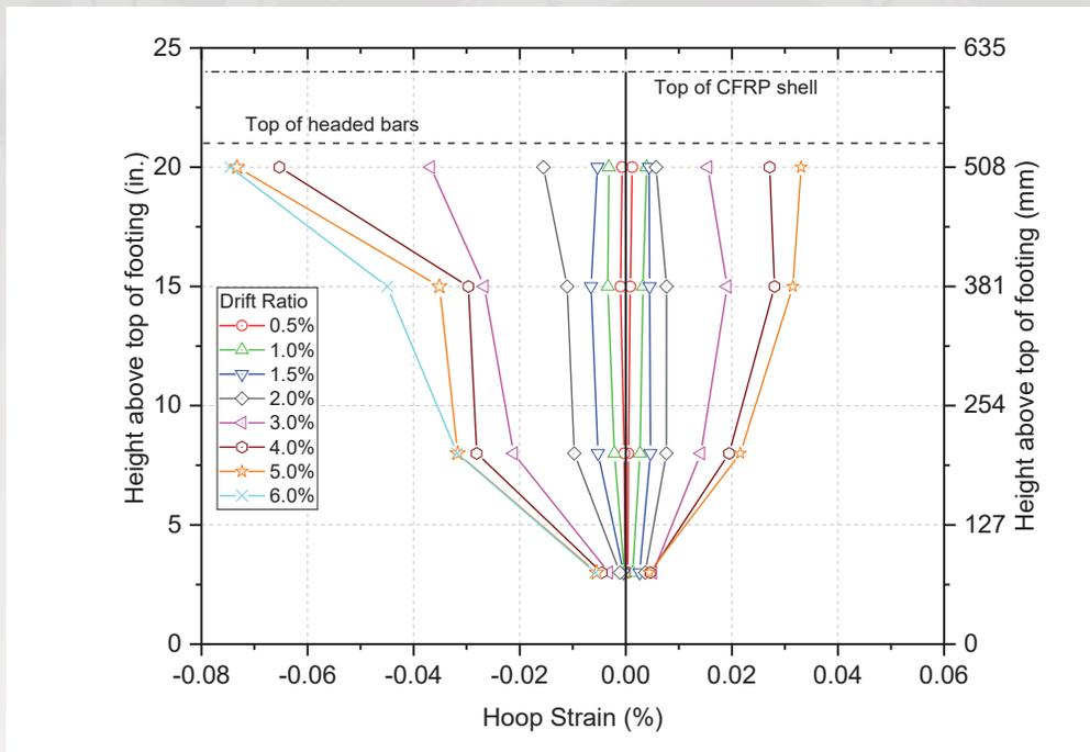
Hoop strain in CFRP shell of modern code compliant wall pier repair
