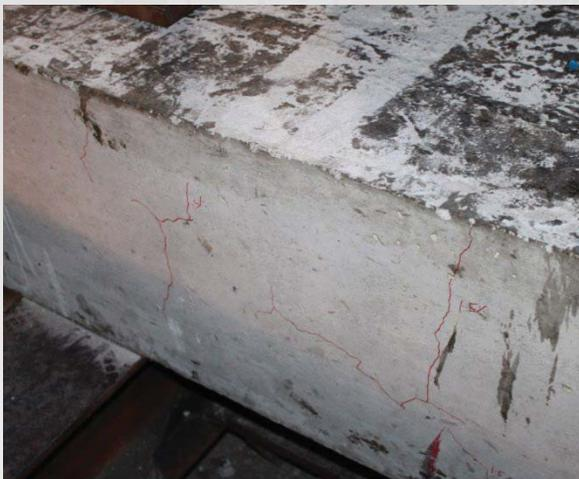
Footing crack at 1.5% drift ratio
