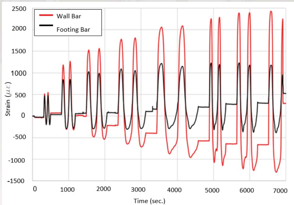
As-built wall pier strain in lap-spliced bars
