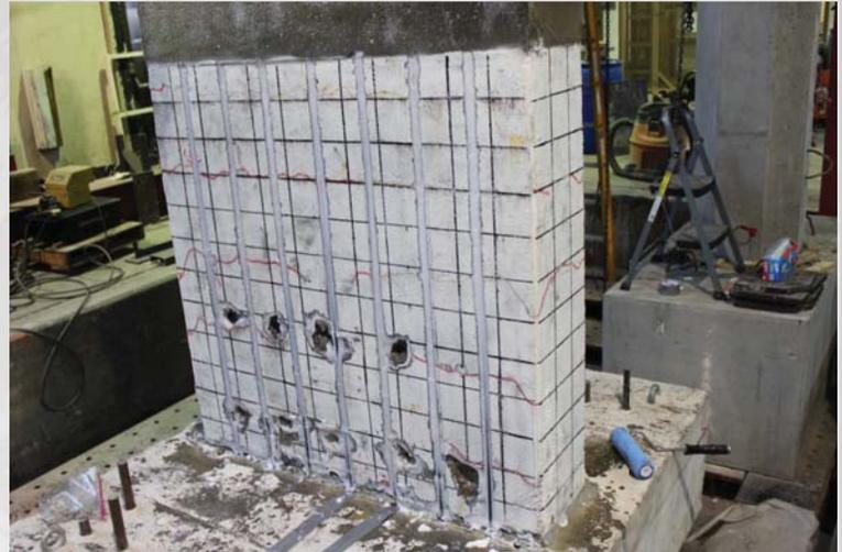
Epoxy coverage of Mild Steel NSM bars
