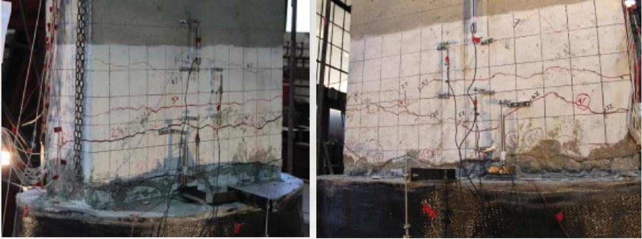
Experimental observation of specimen MCRP at a 5% drift ratio
