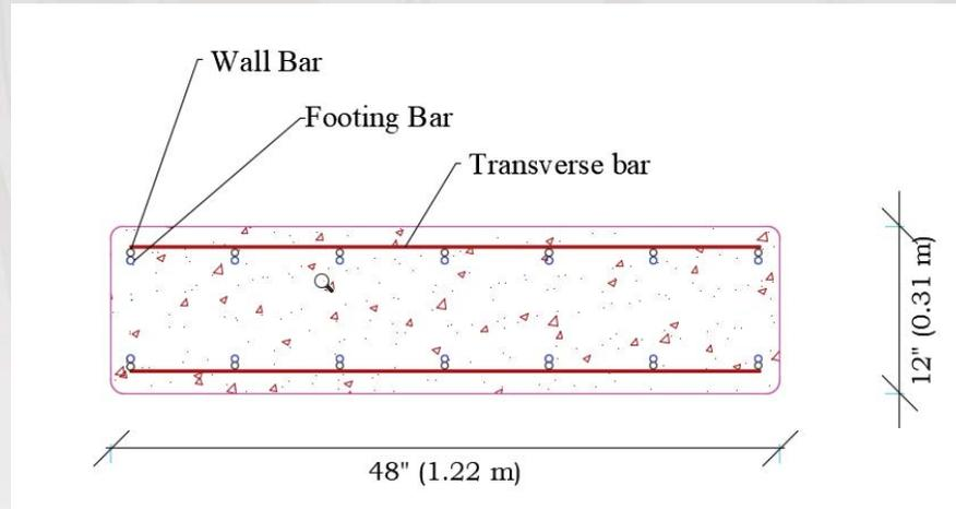
As-built (AB) specimen dimensions and steel reinforcement:
