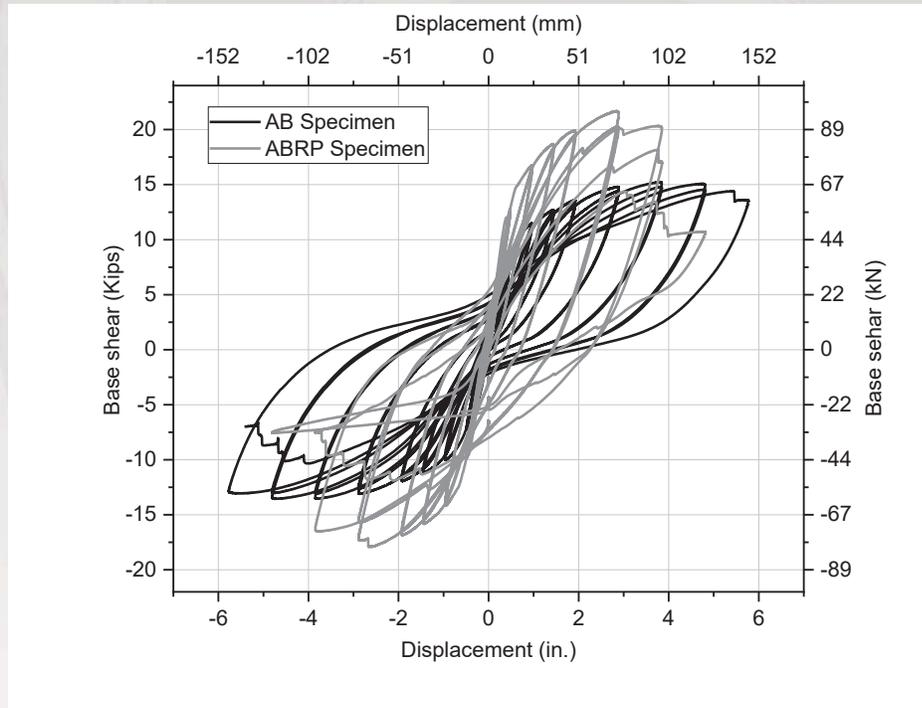
Comparison of **As-built** and **As-built Repair** hysteresis
