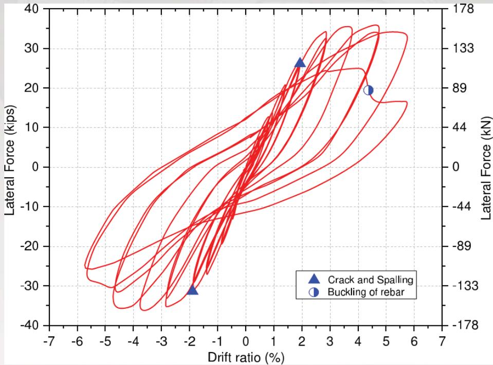
Hysteresis of repaired specimen MCRP
