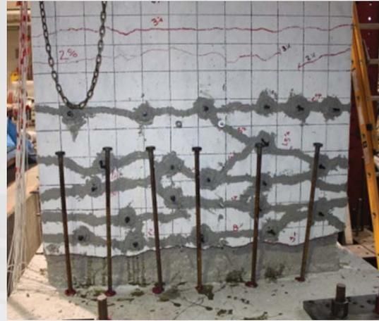
Epoxy injection of cracks for specimen MCRP
