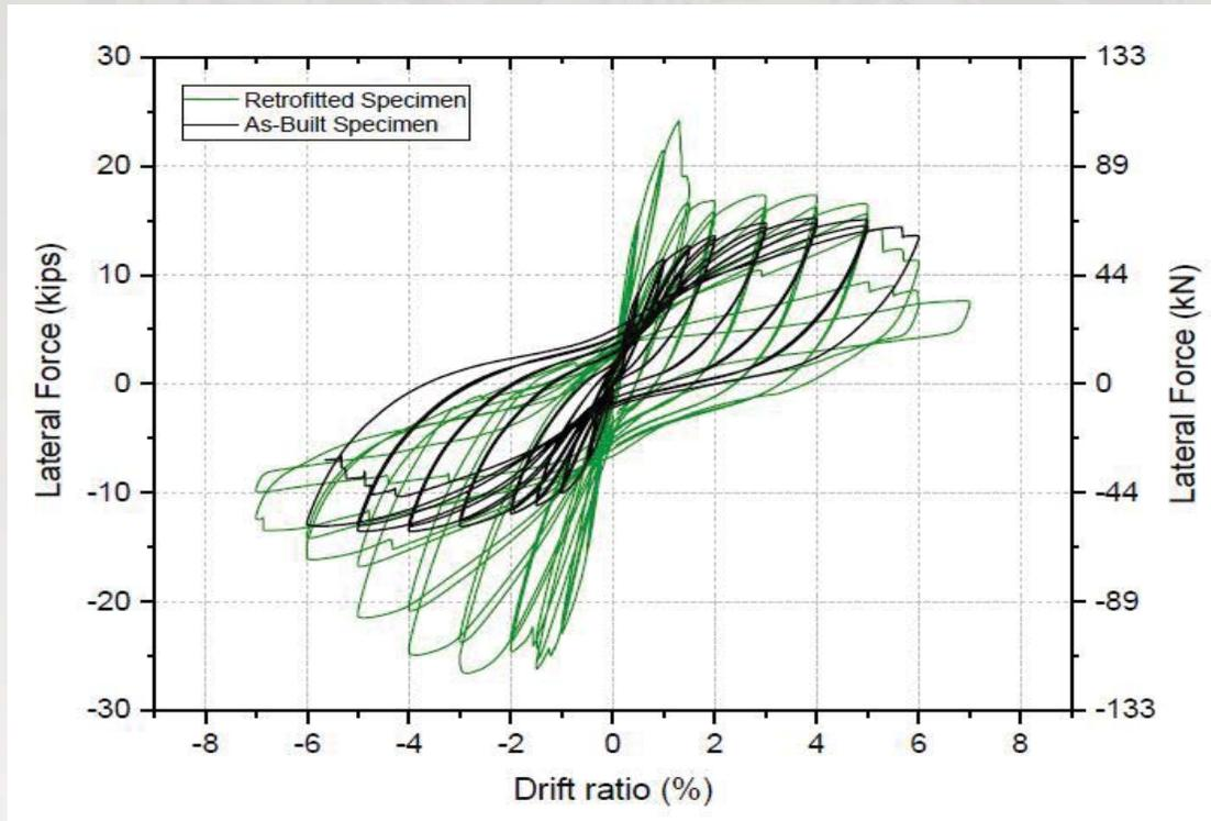
Comparison of hysteresis curves of as-built specimen AB and retrofit specimen R2
