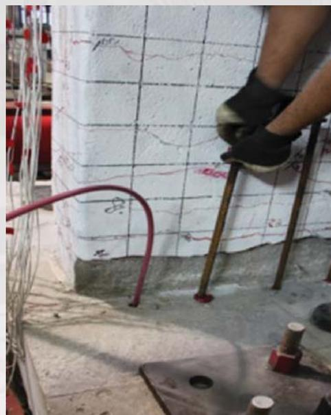
Headed steel bar installation process: (left) drilling holes; (right) headed bar placement for specimen MCRP
