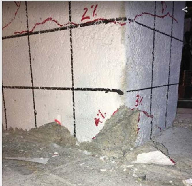
Spalling at 4% drift of as-built wall pier
