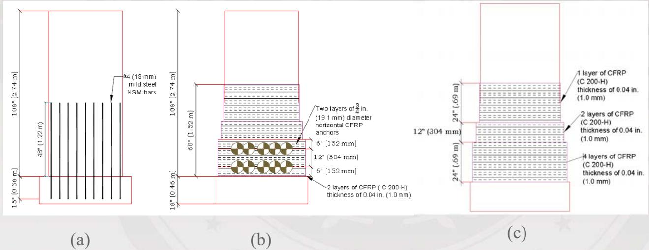
Repair of specimen ABRP: (a) steel NSM bars; (b) horizontal CFRP anchors; (c) hoop direction CFRP jackets
