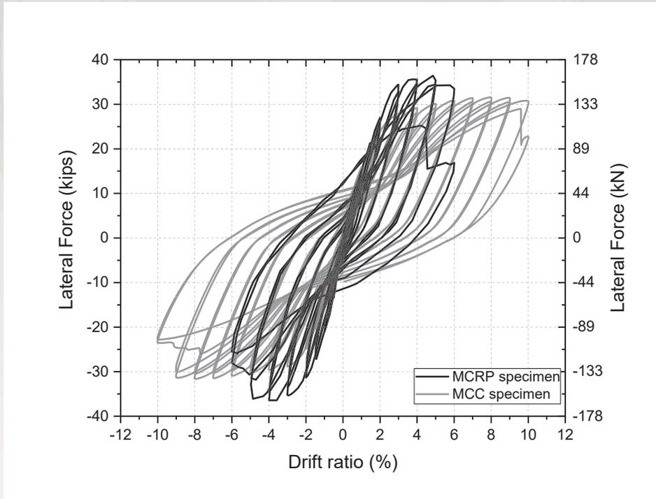
Comparison of Modern Code Compliant and Modern Code Compliant Repair hysteresis
