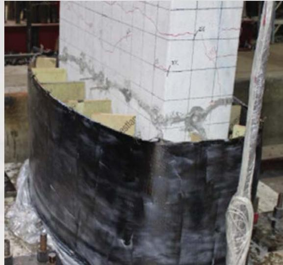
CFRP donut formation: (left) shell formation with precut aluminum foil;
