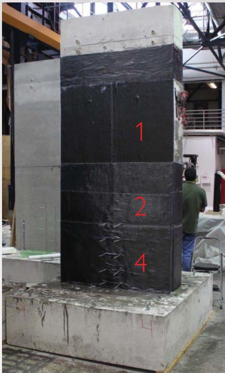
CFRP on each wall face:
