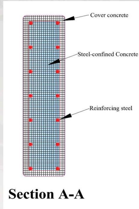
OpenSees fiber model of modern code compliant concrete wall pier
