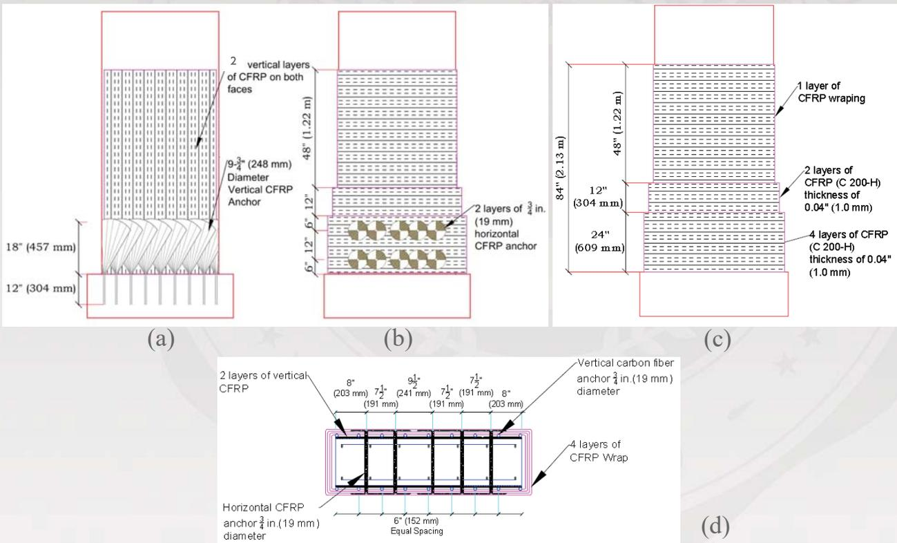
Retrofit design of wall pier R1: (a) 18 vertical CFRP sheets and vertical CFRP anchors; (b) 10 transverse (horizontal) CFRP anchors; (c) 4+2+1 hoop direction CFRP jackets; (d) wall cross-section at bottom 24 in.
