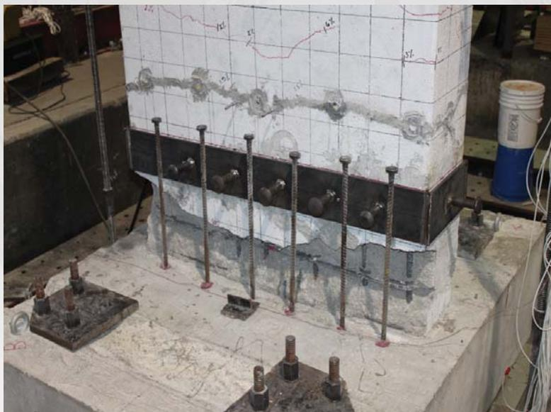
Steel collar with shear studs
