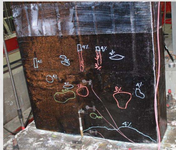
East face CFRP jacket debonding at 4.0% drift ratio
