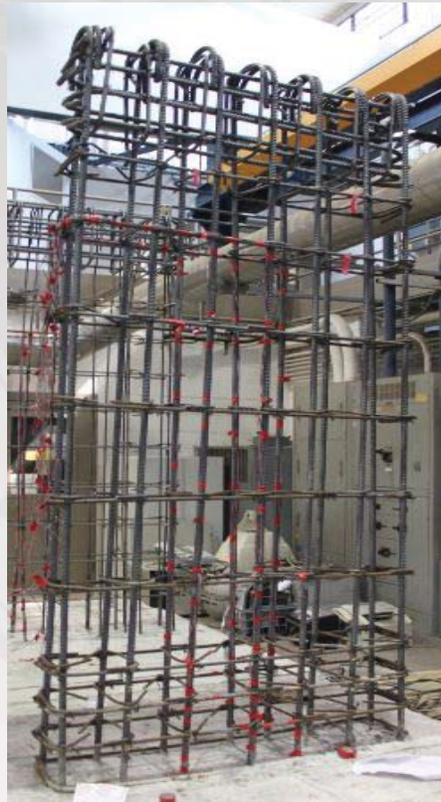
Modern code compliant wall pier reinforcement
