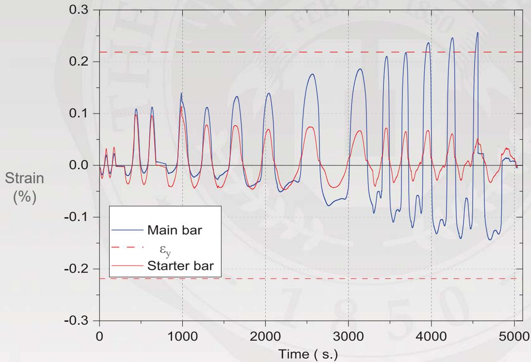
Retrofitted specimen R2 lap-splice strain in the footing and wall bars
