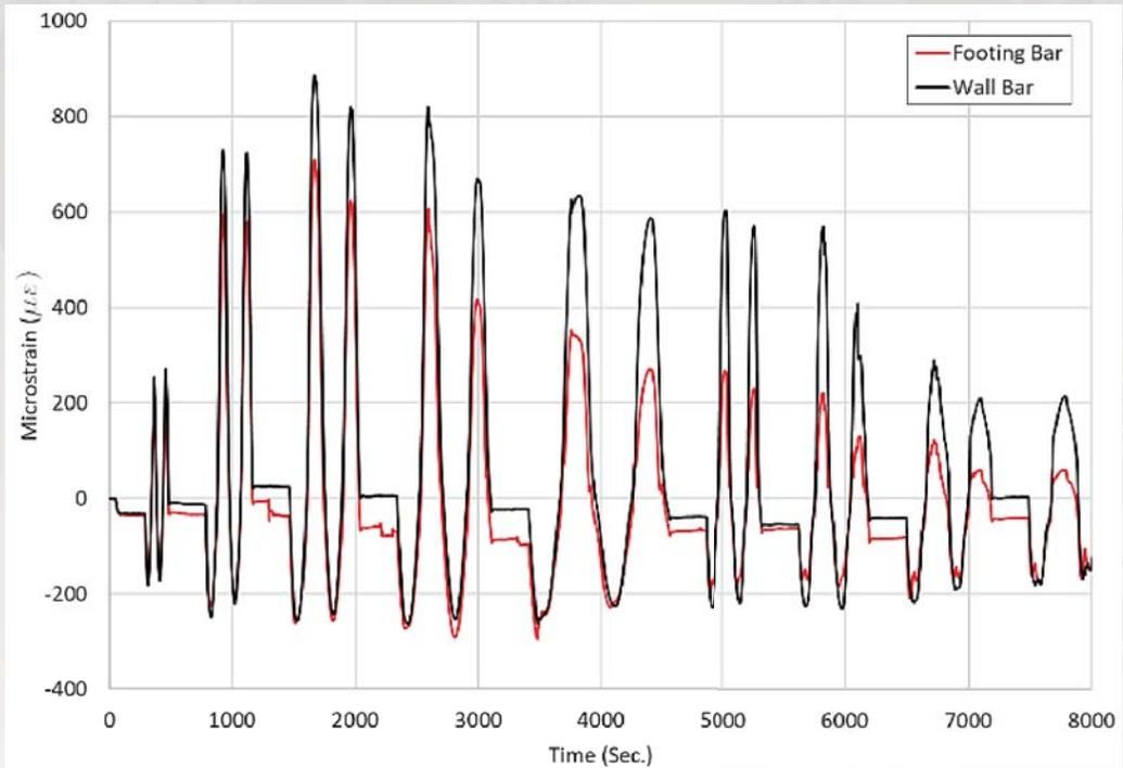
Retrofitted specimen *RI* lap-splice strain in the footing and wall bars
