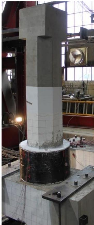
Figure 6. Seismic repair of a column to footing joint using CFRP composite donut.
