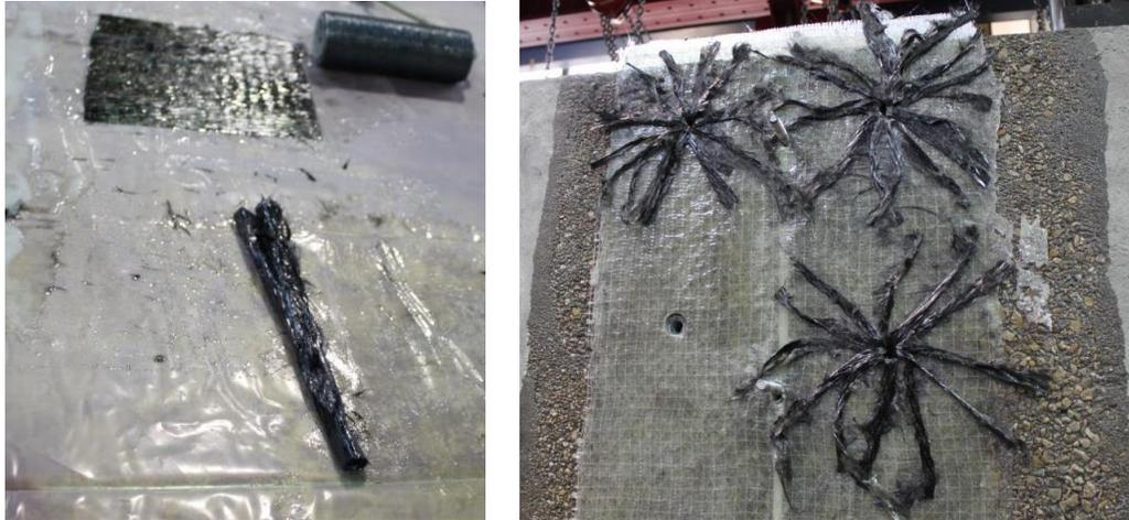
Figure 7. CFRP anchor and application to precast concrete wall strengthening.
