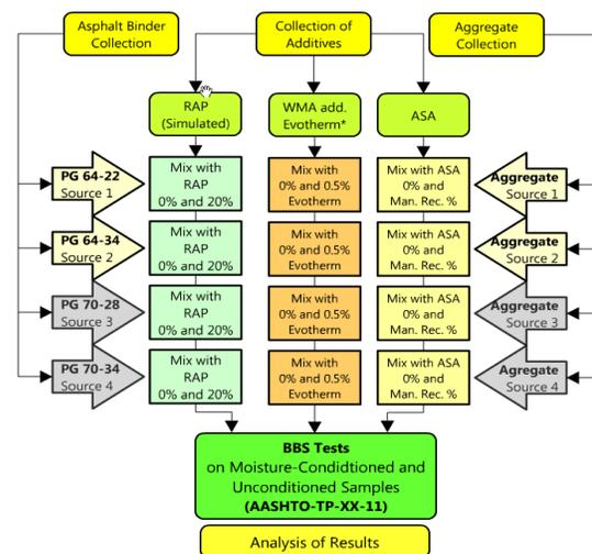
Figure 3 Work flow and plan for BBS tests
