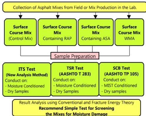
Figure 2 Work flow and plan for testing mixes
