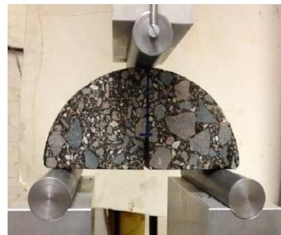
Figure 1 A photographic view of SCB test
