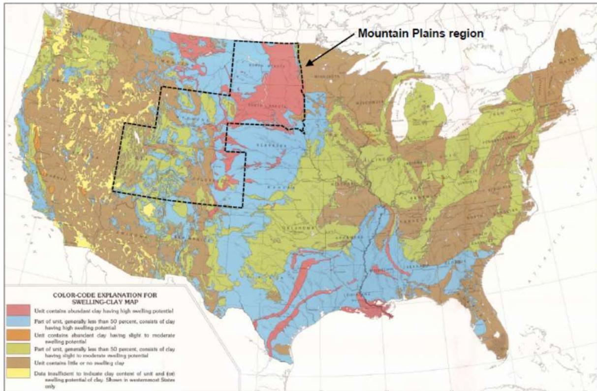
**Figure 1.** Map of expansive soils in the continental United States (adapted from Olive et al. 1989). Areas in red, blue, orange, and green have > slight to moderate swelling potential, and thus the potential for damage transportation infrastructure.
