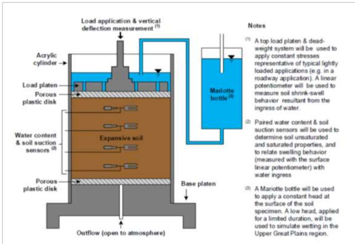
**Figure 2.** Preliminary conceptual diagram of proposed testing apparatus. A 12-in diameter specimen is proposed to minimize boundary effects.
