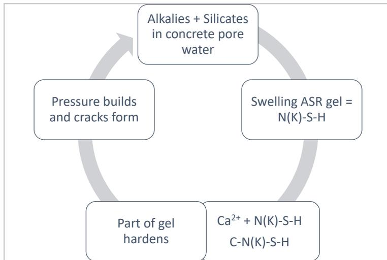
**Figure 1.** Illustration of viscous cycle of ASR damage
