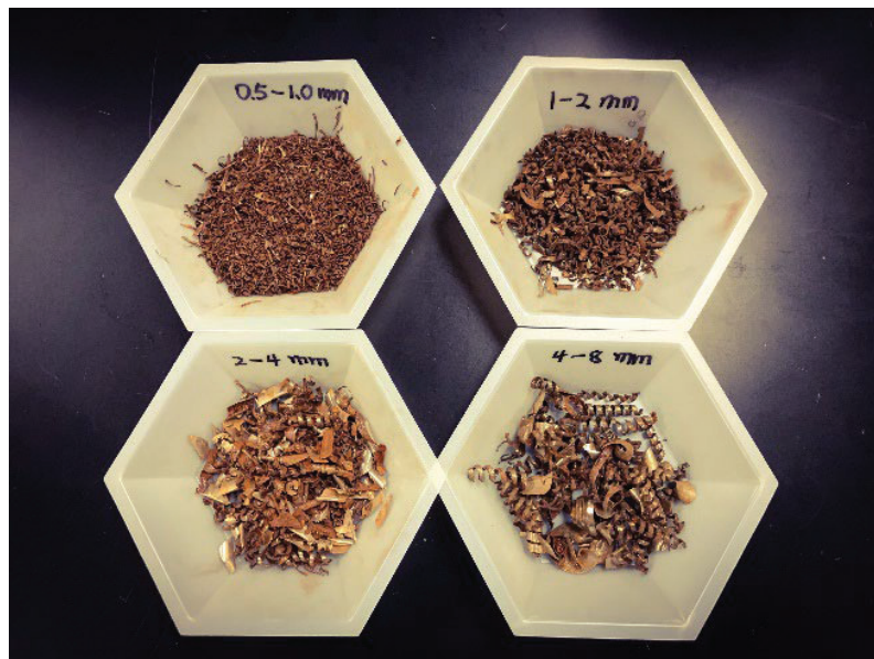
Steel Chips (0.5-1, 1-2, 2-4 and 4-8 mm)
