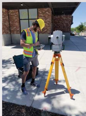
Maptek I-Site 8820 Terrestrial LiDAR Scanner – Pedestrian Access Ramps & Pavement Distress
