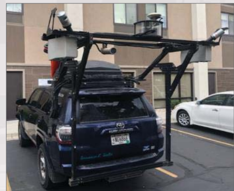
Mandli Communications Mobile LiDAR Vehicle - Asset Management
