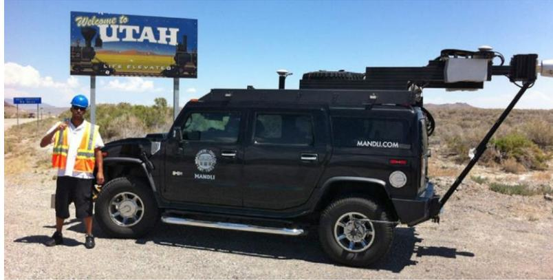
**Figure 3.** Sensors on the UDOT Mandli vehicle [12]
