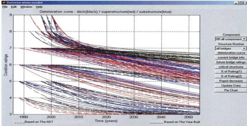
*Fig. 2 Bridge deterioration patterns for a number of bridges in the City and County of Denver*
