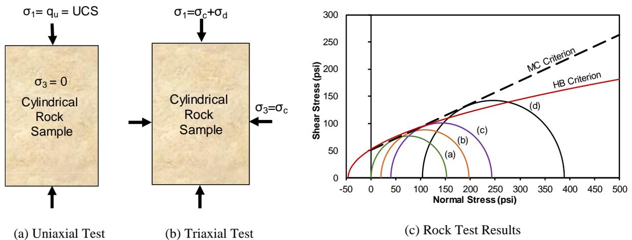
Figure 2. (a) Stress state at uniaxial compressive test, (b) stress state at triaxial compressive test, and (c) a combination of uniaxial and triaxial test results including two failure envelopes.
