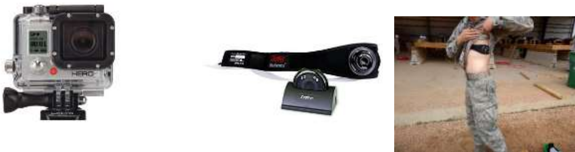
Figure 1: Equipment used to collect and monitor physiological data on-site (L). Volunteer wearing bio-harness while performing construction activities (R).
