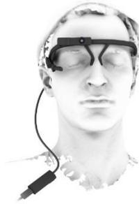
*Figure 1. Pupil Lab's Wearable Eye-Tracker with World Camera*
