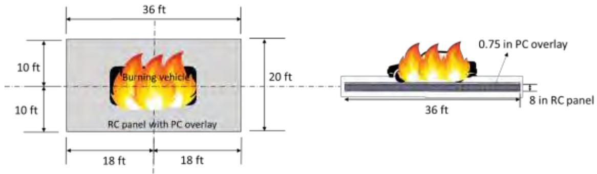
**Figure 4 A vehicle fire test on a large RC panel overlaid by PC**
