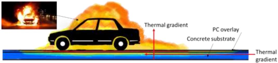
**Figure 2 Thermal gradient of a bridge deck under a vehicle fire**
