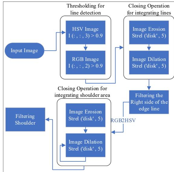
Figure 6. The Process of Filtering Images for Shoulder Width Detection
