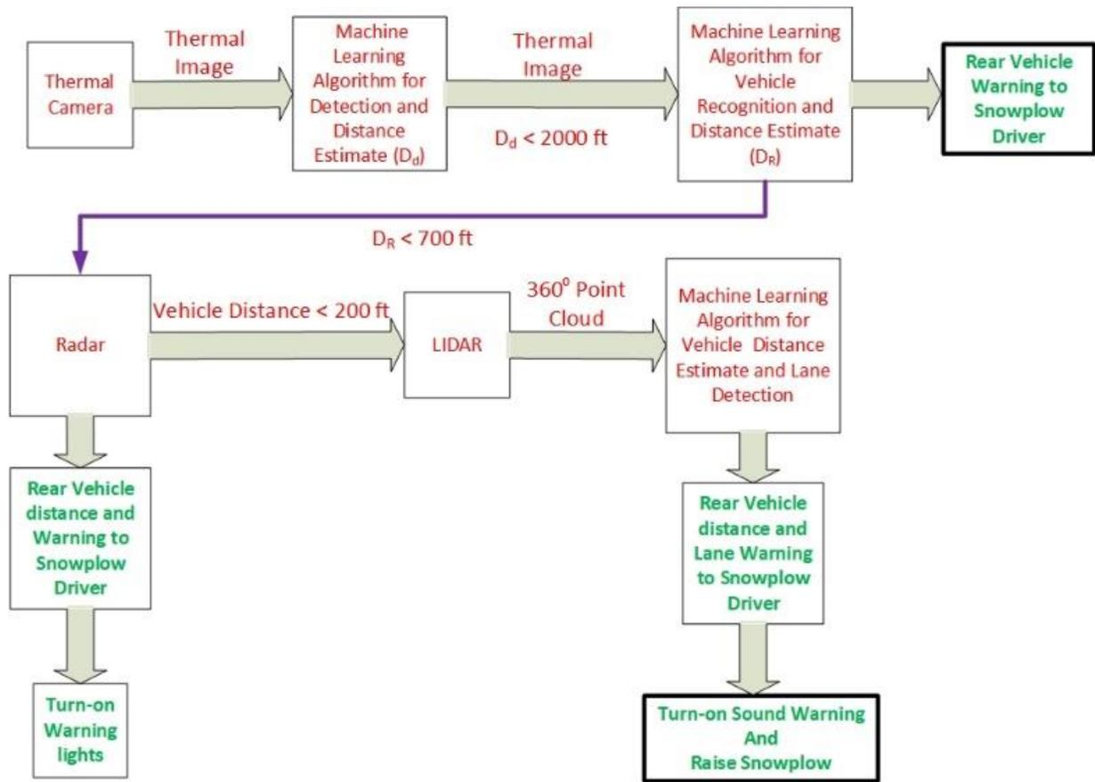
**Fig 6. Software Framework of the Prototype Device**
