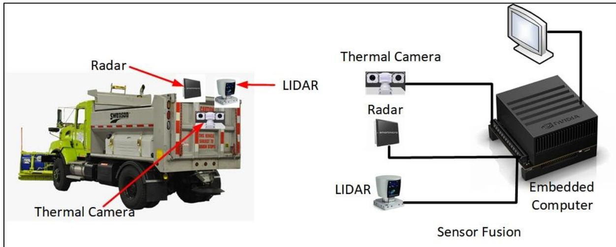
**Fig 5. Hardware Prototype**
