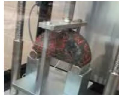
Figure 3. SCB Test in Progress (SDSU’s Asphalt Laboratory)
