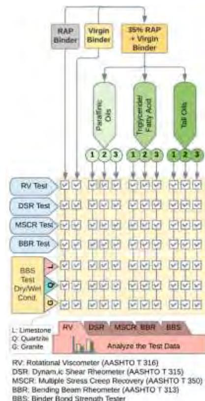
Figure 1. Workflow and Test Matrix for Binder Study
