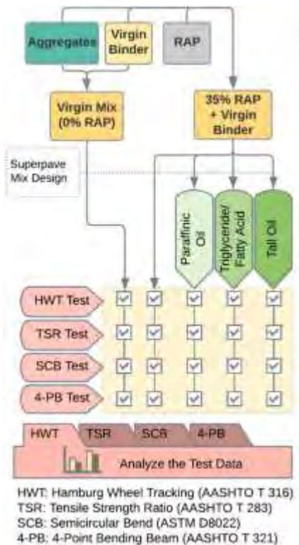
Figure 2. Workflow and Test Matrix for Mix Study
