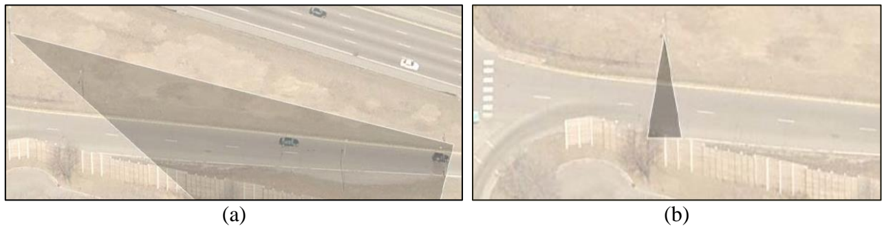
Figure 2. Arrangements of Radar Sensors (a) Queue Length Detection (b) Vehicle Counting
