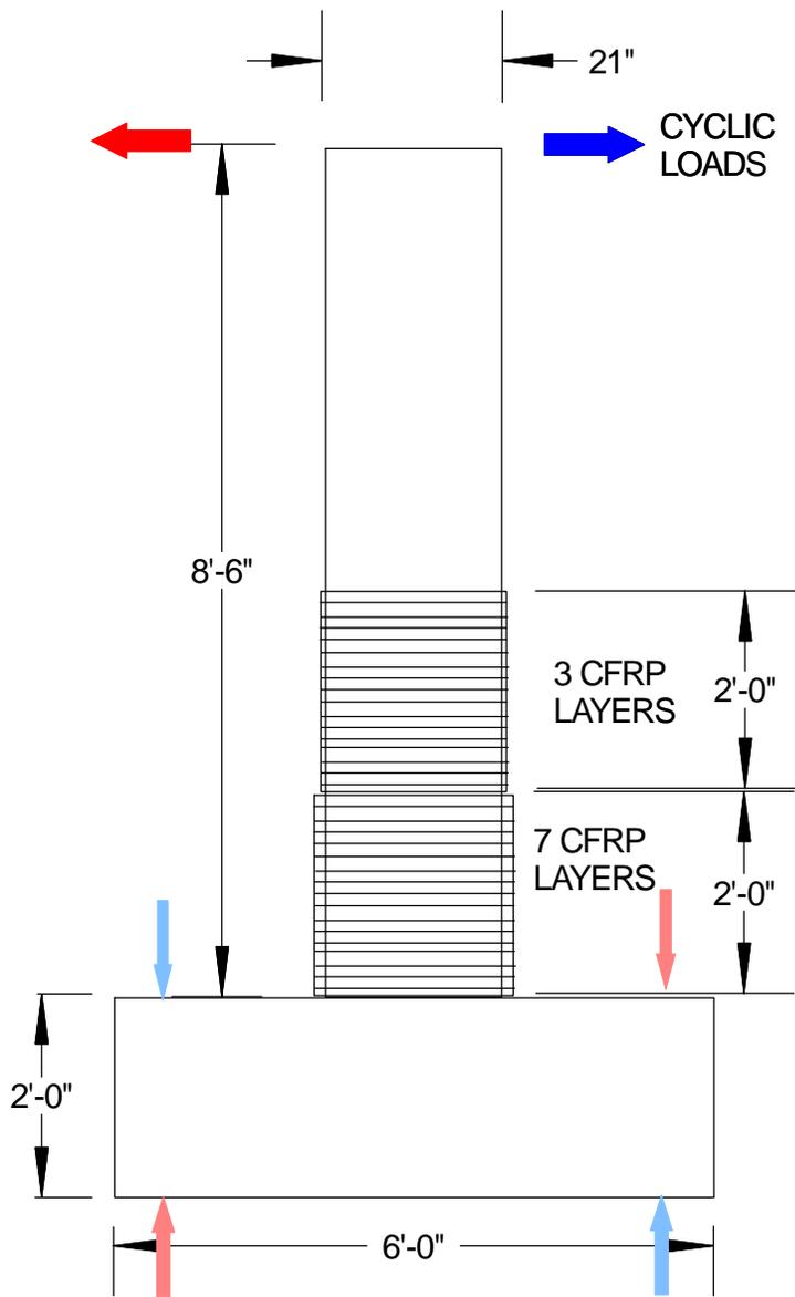
Figure 2. Seismic Retrofit of the column to footing joint using NMB splice sleeves.
