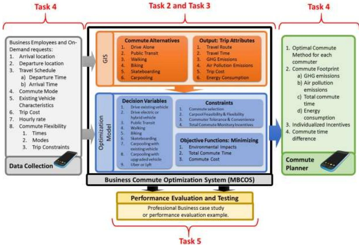
Figure 2. Components of BCOS and Main Research Tasks
