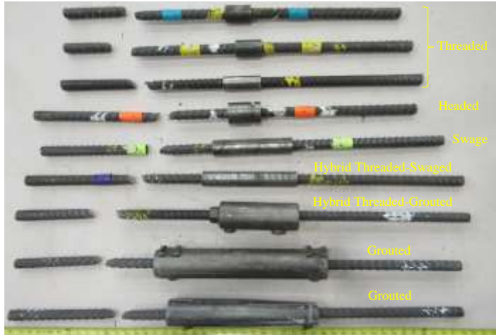
Figure 1. Seismic Couplers Suitable for Incorporation in Precast Columns
